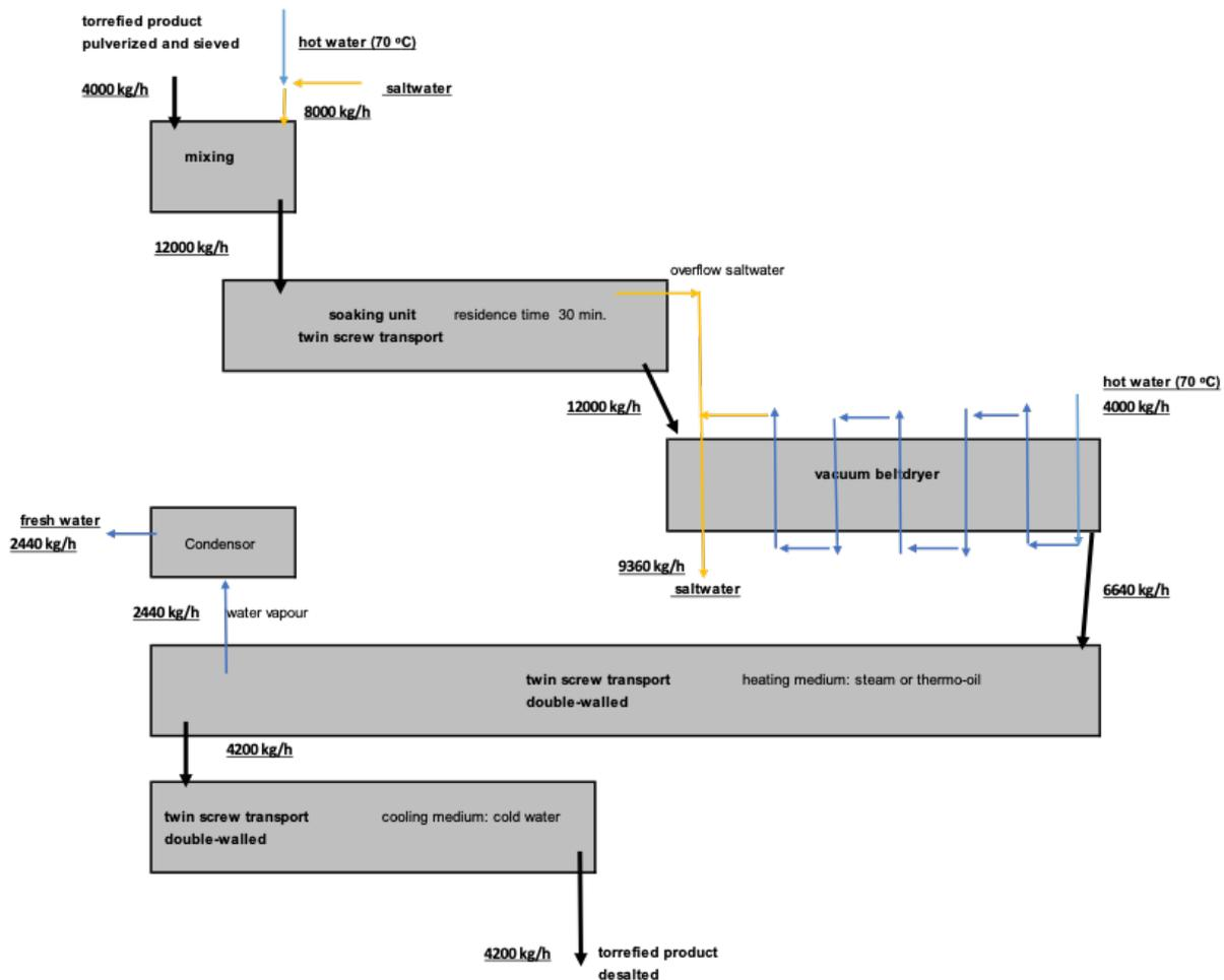
Fig. 1: setup product cleaning process.
